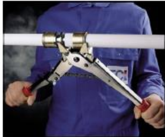
Afb. 22 Axiale persverbinding (bron TeCe)
